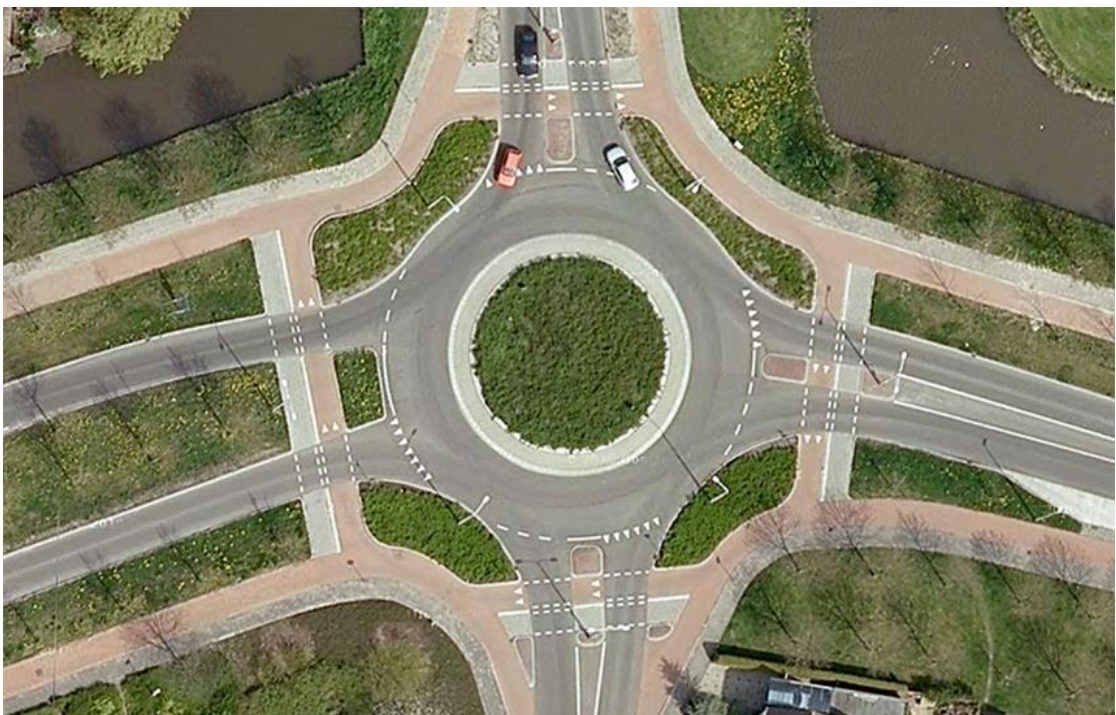
Figure 2: Dutch Style single lane approach example
