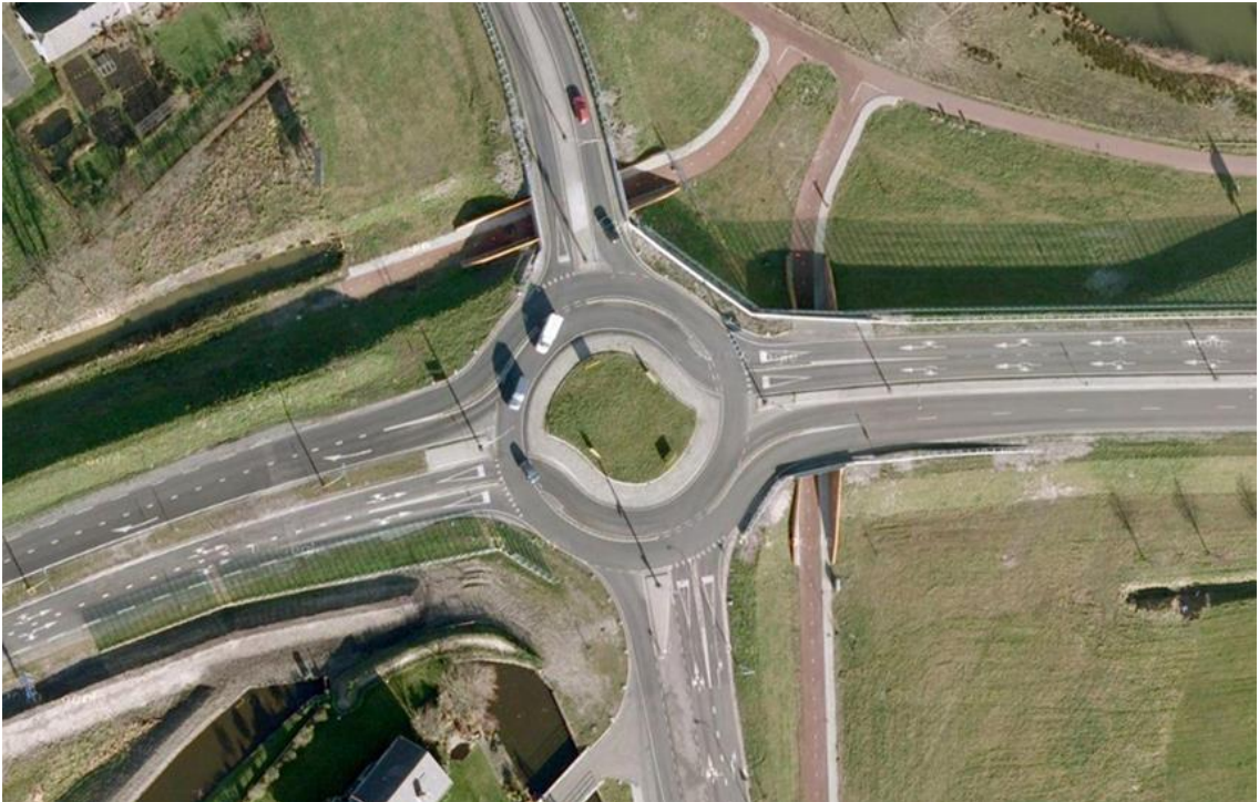
Figure 3: An example of a ‘Turbo Style’ Dutch Roundabout
